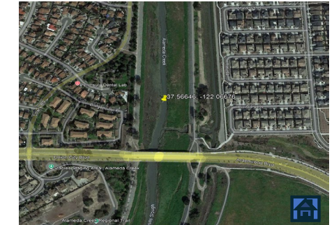
A6 – Ditch. Low to moderate entrenchment, gently sloped, natural bank composition, plane bed, fine bed sediment
