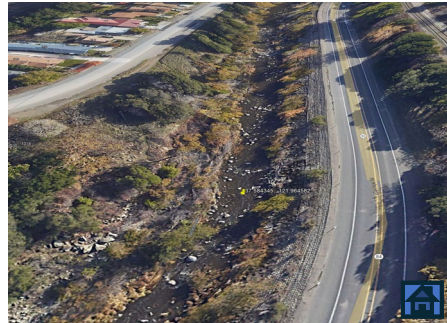
A3 – Naturalizing canal. Deeply entrenched, wide, natural bank composition, strong bed undulations, coarse bed sediment
