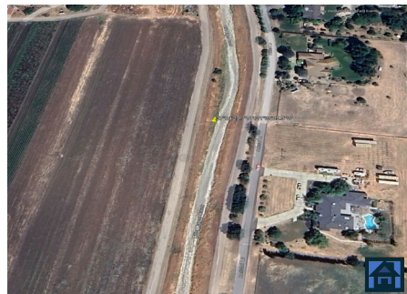
A3 – Naturalizing canal. Deeply entrenched, wide, natural bank composition, strong bed undulations, coarse bed sediment
