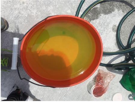
Dye tablet dissolving in 5 gallon bucket of water
