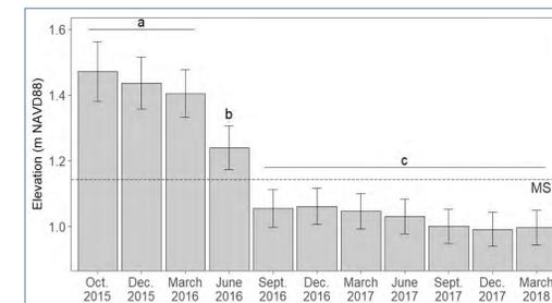
Figure 7: Marsh Mound Early Erosion. Prior to planting experiments and ISP mound planting, many mounds lost about 0.5 m to erosion, indicating the consequence of no pre-breach stabilization planting as designed (see Figure 5A).
