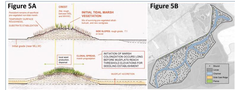
Figure 5: Marsh Mound Design (A) and Constructed Locations (B). The design report (WWR 2007 Figure 13) called for pre-breach vegetation stabilization (Figure 5A, drawn by Peter Baye) of the ~500 mounds distributed throughout the site (Figure 5B).
