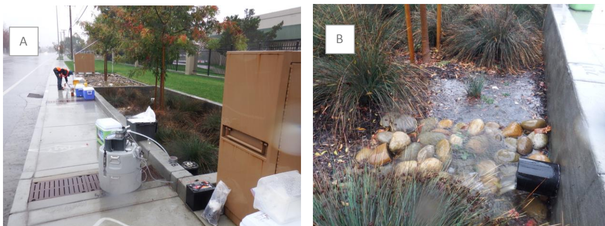
Figure 3. A) ISCO pumping sampler set up at the surface-loaded TWF inlet; SFEI staff member checking Cole Parmer peristaltic pumping sampler at subsurface-loaded tree well filter outlet. B) Stormwater runoff flowing into surface-loaded tree well filter during a monitored storm event.
