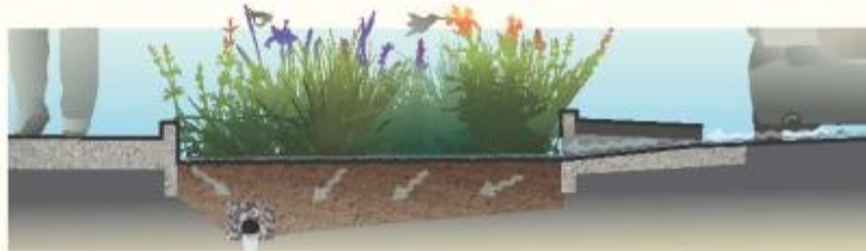
Plants like these in a Portland stormwater planter help catch and slow runoff while providing habitat for pollinators and birds. Photo by Lisa Owens Viani.
